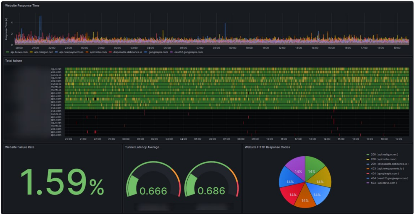
Dependency health dashboard (proxy/API checker). Pythonic checker monitoring critical external dependencies (payment, mail, auth providers) — response time, failure rate (1.59% shown), tunnel latency and HTTP status mix.
